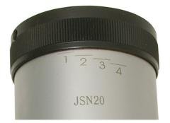
The tapping head has adjustable torque settings to prevent tap breakage. Utilising a large knurled knob to easily adjust the torque.
