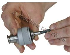
Insert machine tap and locate the square of the tap with the square at the rear of the collet
